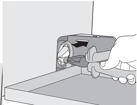
6. When no more water comes out, unscrew the pump cover by turning it anti-clockwise, using pliers, and remove the filter. Always keep a rag nearby to dry up any water spillages when removing the cover.
